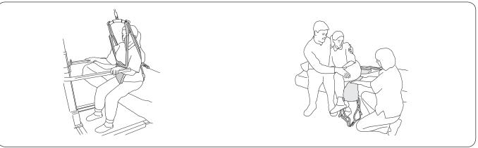
Lower the patient down into a sitting position. Unhook the rear suspension straps and front suspension straps from the sling bar. Loosen the rear suspension straps from the loop straps.
