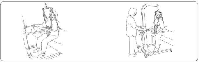
Before the patient is raised from the sitting position: Have the patient move as far forward on the seated surface and bring their feet as far back on the floor as needed to stand up comfortably. Raise the lift slightly, so that tension is applied to the straps without the patient's seat rising from the underlying surface, while ensuring that strap tension on the upper body is as comfortable as possible for the patient.
