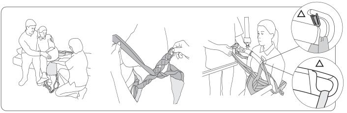
The starting position for using LiftPants sling is the sitting position. The patient leans to one side to enable the caregiver to position LiftPants sling directly under the seat. Place LiftPants sling as far as possible under the patient, with the marking label facedown and towards the back of the seat.
